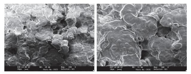
Fig. 2. Scanning electron photomicrograph showing calcium alginate and starch beads coated with chitosan layer at magnification of: a) 200× and b) 500×
