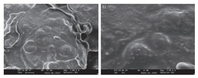
Fig. 3. Scanning electron photomicrograph showing Hi-maize resistant starch granules on the surface of calcium alginate and starch beads coated with chitosan layer at magnification of: a) 1000× and b) 3000×
