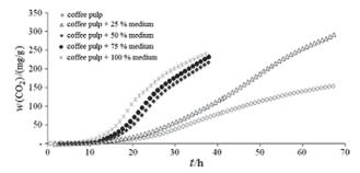
Fig. 2. CO<sub>2</sub> production during SSF of coffee pulp by *A. tamarii* V12307 using five different dilutions of culture medium
