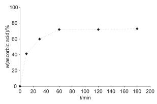
Fig. 6. Kinetic release profile of AA xerogel expressed as percentage of AA relative to the total loaded amount
