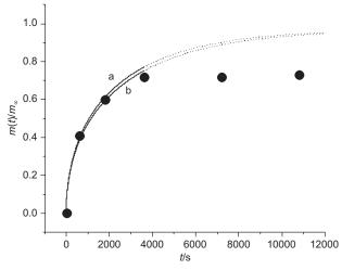
**Fig.** 7. AA release from xerogel. Dots: experimental results. The lines represent two release curves estimated from Robinson *et al.* (11) using  $D_{\text{eff}}$  values of  $1.90 \cdot 10^{-7}$  and  $1.75 \cdot 10^{-7}$  cm<sup>2</sup>/s, respectively
